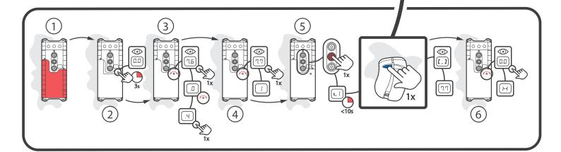
To pair each transmitter, select parameter 7.7 and press the STOP button when . is present on the TS 971 display. Within 10 seconds of this, press the transmitter button you wish to pair to the door controller.
