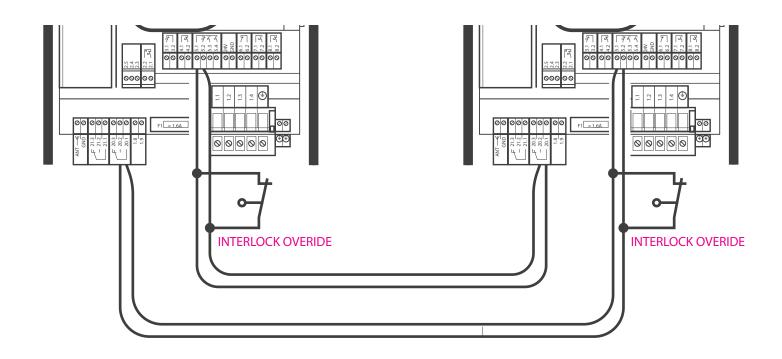
Interlocking both TS 971's only allows one door to be opened at a time.
