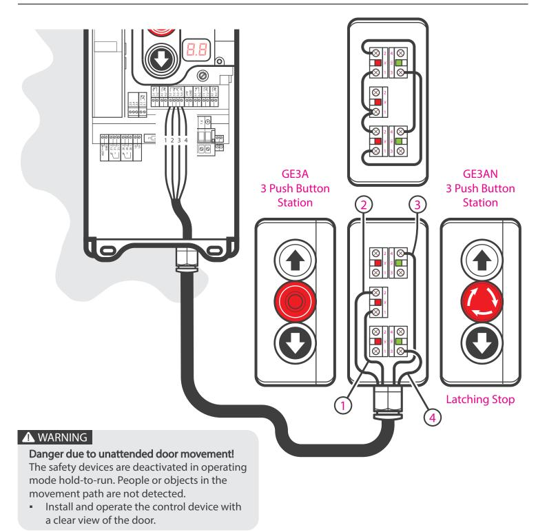
The Push Button Station must be in clear view of the door, and should be operated by trained users ONLY, or a photocell and safety edge must be fitted to detect persons or obstacles standing on the floor to one side of the door.
